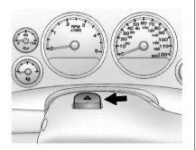
(Hazard Warning Flashers): Press this button located on top of the steering column, to make the front and rear turn signal lamps flash on and off. This warns others that you are having trouble. Press again to turn the flashers off.
