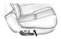
2. Lift the lever, on the outboard side of the seat, to release the seatback.
