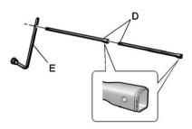
Assemble the two jack handle extensions (D) and wheel wrench (E) as shown.
