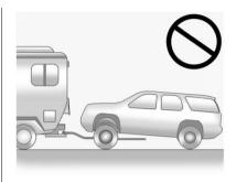
Notice: Towing an all-wheel-drive vehicle with all four wheels on the ground, or even with only two of its wheels on the ground, will damage drivetrain components. Do not tow an all-wheel-drive vehicle with any of its wheels on the ground.
