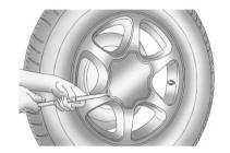
If the wheel has a center cap that covers the wheel nuts, place the chiseled end of the wheel wrench in the slot on the wheel and gently pry the cap out.
