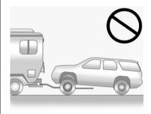
Notice: If a two-wheel-drive vehicle is towed with the rear wheels on the ground, the transmission could be damaged.
