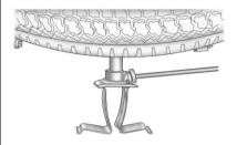
Attach the jack handle, extension, and wheel wrench to the jack and place it (with the wheel blocks) under the vehicle toward the front of the rear bumper.
