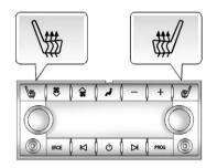
The buttons are on the Rear Seat Audio (RSA) panel on the rear of the center console.
