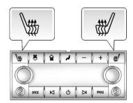
The buttons are on the Rear Sear Audio (RSA) panel on the rear of the center console.
