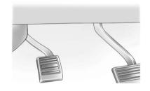
Set the parking brake by holding the regular brake pedal down, then pushing down the parking brake pedal.
