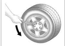
Use the wheel wrench to loosen all the wheel nuts. Turn the wheel wrench counterclockwise to loosen the wheel nuts. Do not remove the wheel nuts yet.
