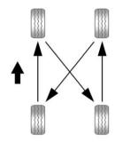
When rotating the vehicle's tires, always use the correct rotation pattern shown here.
