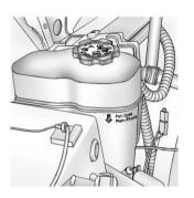
The coolant surge tank is located in the engine compartment on the passenger side of the vehicle. See *Engine Compartment Overview on page 10-6* for more information on location.
