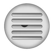
The interior temperature sensors located in the headliner above the driver side seat and if equipped, in the headliner above the second row seats measure the temperature of the air inside the vehicle.
