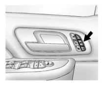
The controls on the driver door are used to program and recall memory settings for the driver seat, outside mirrors, power steering column, and the adjustable throttle and brake pedals.
