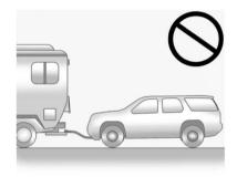
Notice: If a two-wheel-drive vehicle is towed with all four wheels on the ground, the transmission could be damaged. The repairs would not be covered by the vehicle warranty. Do not tow a two-wheel-drive vehicle with all four wheels on the ground.
