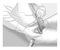
If the belt stops before it reaches the buckle, for lap-shoulder belts with cinching latch plates, tilt the latch plate and keep pulling the safety belt until it can be buckled.
