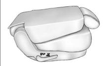
The seatback will fold forward to create a flat load floor.
