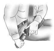
Push the latch plate into the buckle until it clicks. If you find that the latch plate will not go fully into the buckle, see if you are using the correct buckle.
