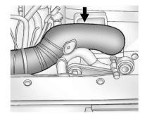
With the coolant surge tank pressure cap off, start the engine and let it run until the upper radiator hose can be felt getting hot. Watch out for the engine cooling fan.
