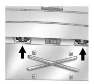
Remove the two screws holding each of the license plate lamps to the molding that is part of the liftgate.
