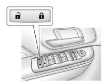
(Unlock): Press to unlock the doors.
