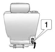
Lift the release lever "1," on the bottom rear of the seatback on the outboard side of the seat, and the seatback folds forward.
