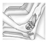
For third row seating positions, with cinching latch plates, tilt the latch plate to adjust the belt if needed.
