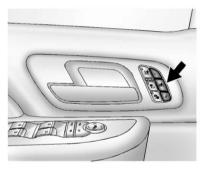
The controls on the driver door are used to program and recall memory settings for the driver seat, outside mirrors, power steering column, and the adjustable throttle and brake pedals.
