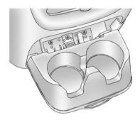
Pull downward on the cover, in the rear floor console to access the cupholders.
