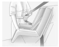
4. For passenger seating positions with a lap-shoulder belt and a free-falling latch plate, pull the rest of the shoulder belt all the way out of the retractor to set the lock. When installing a child restraint using a lap-shoulder belt and a cinching latch plate, skip Step 4 and proceed to Step 5.
