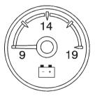
When the engine is not running, but the ignition is on, this gauge shows the battery's state of charge in DC volts.
