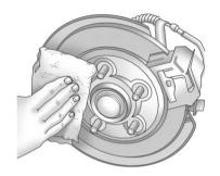
Remove any rust or dirt from the wheel bolts, mounting surfaces and spare wheel.
