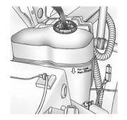
Fill the coolant surge tank with the proper mixture to the FULL COLD mark.
