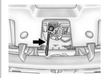
2. Then go to the front of the vehicle and locate the secondary hood release, near the center of the grille.
