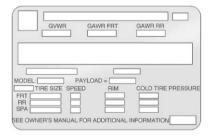
A vehicle specific Certification/ Tire label is found on the rear edge of the driver door. The label shows the size of your vehicle's original tires and the inflation pressures needed to obtain the gross weight capacity of your vehicle. This is called Gross Vehicle Weight Rating (GVWR). The GVWR includes the weight of the vehicle, all occupants, fuel and cargo.
