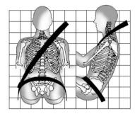
Sit up straight and always keep your feet on the floor in front of you. The lap part of the belt should be worn low and snug on the hips, just touching the thighs. In a crash, this applies force to the strong pelvic bones and you would be less likely
