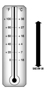
Cold Temperature Operation: In an area of extreme cold, where the temperature falls below -29°C (-20°F), an SAE 0W-30 oil should
