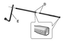
Assemble the two jack handle extensions (D) and wheel wrench (E) as shown.
