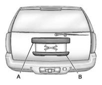
On vehicles with a liftglass, press the button on the underside of the license pocket applique (A) to open it. The liftglass can also be opened by pressing on the RKE.
