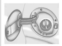
The tethered fuel cap is located behind a hinged fuel door on the driver side of the vehicle. If the vehicle has E85 fuel capability, the fuel cap will be yellow and state that E85 or gasoline can be used. See Fuel E85 (85% Ethanol) on page 9-59.
