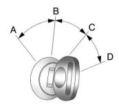
The ignition switch has four different positions.
