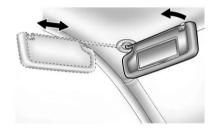
Pull the sun visor down to block glare. Detach the sun visor from the center mount to pivot to the side window, or to extend along the rod, if available.
