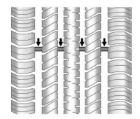
Treadwear indicators are one way to tell when it is time for new tires. Treadwear indicators appear when the tires have only 1.6 mm (1/16 in) or less of tread remaining. Some commercial truck tires may not have treadwear indicators. See *Tire*
