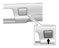
To remove the spare tire lock, insert the ignition key, turn it clockwise and then pull straight back.
